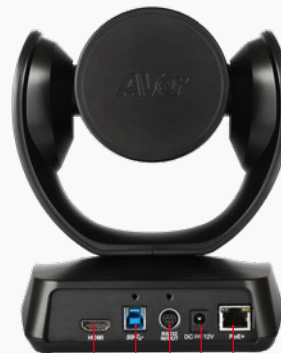
HDMI out USB 3.1 type-B RS232 in/out DC 12V LAN for IP streaming and PoE+
