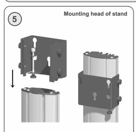
Slide the head of the stand from the top downwards by using the T-ducts on both sides of the column. Tight the knobs on the right and left-hand side of the head to fix on a specific height.
