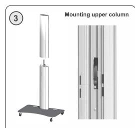
Place the upper column of the stand (cable duct closed) carefully on the bottom column. Use the latch to secure upper column of the stand to the bottom column.
