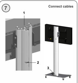
The cables can be guided through the cable duct(s). The cables can come out of the ducts at the top of the column (1) or out of the cover gab (2). The other side of the cables can come out of the bottom end of the column (3). All cable ducts have to be closed.
