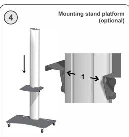
Slide the stand platform from the top downwards by using the T-ducts on both sides of the column. Tight the knobs on the right and left hand site of the platform to fix on a specific height.
