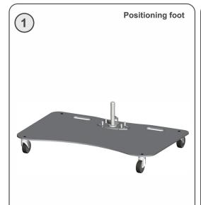
Place the foot on the right position. Activate the wheel brackes (front wheels).
