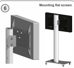
a bracket with three coupling boxes has to be mounted at the back of the flat screen (see specific mounting instructions flat screen brackets)
