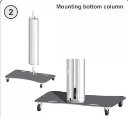
Place the bottom column of the stand (cable duct closed) carefully on the foot plate. Use the latch to secure bottom column to the foot.
